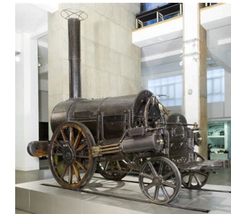
Stephenson's Rocket - the first steam railway engine
